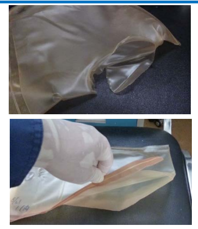
Fig.2 Resin bags after the test (top: outside bag, bottom: inside bag)
