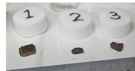
⑥ Scattered material collected from the floor in front of the hood
