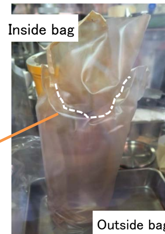
② Resin bags after the burst
